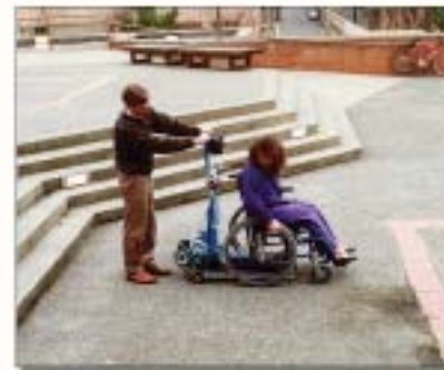
Attach the Stair-Trac to the wheelchair, recline the passenger and move them to the stairway.
